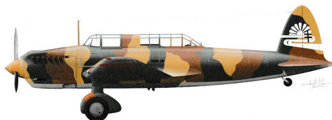
A Kawasaki Ki-32 light bomber of the 16th Hiko Sentai, 9th Hiko Dan. Due to their light handling, the Ki-32 was preferred by pilots over the similar Mitsubishi Ki-30. However, the inline engine frequently overheated and – due to its liquid cooling – was vulnerable to combat damage. (Artwork by Luca Canossa)
